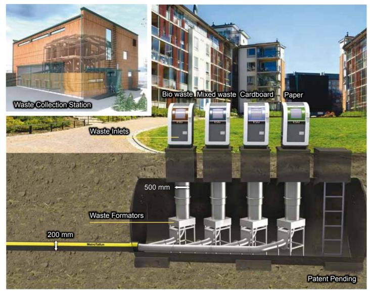
The MetroTaifun system consists of waste inlets which are connected with piping to the central waste collection station. A modular layout allows for easy and efficient installation.
