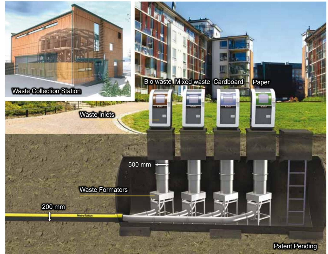
The MetroTaifun system consists of waste inlets which are connected with piping to the central waste collection station. A modular layout allows for easy and efficient installation.
